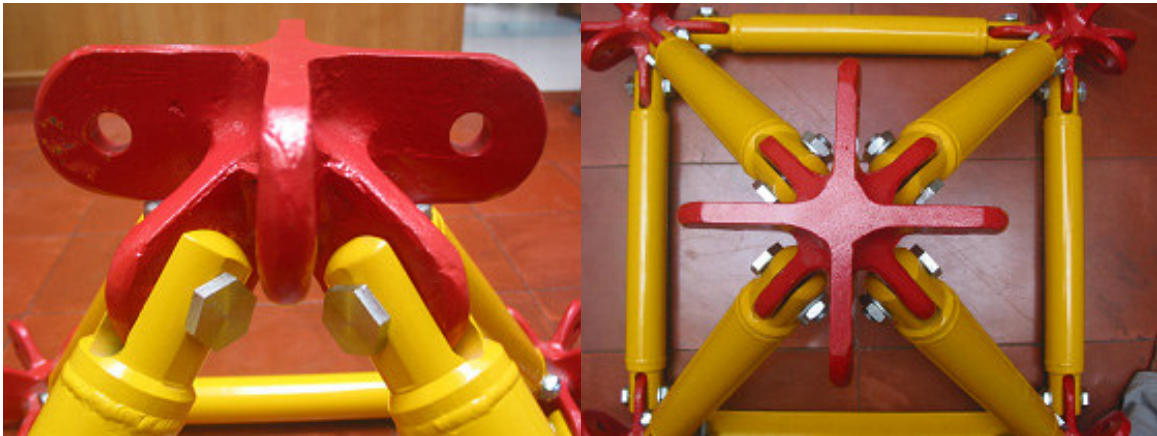
Figure 4. Finished steel cast sample with boltholes
