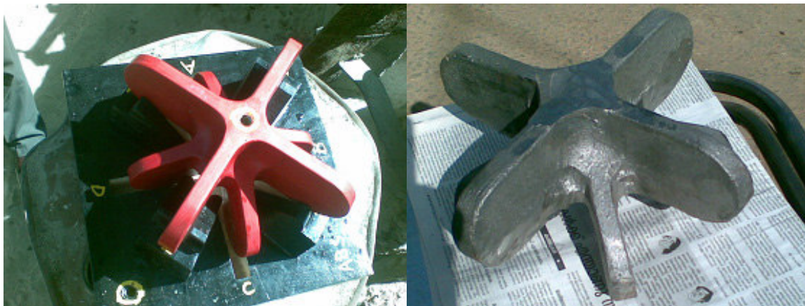
Figure 3. Cast wooden pattern and steel cast sample
